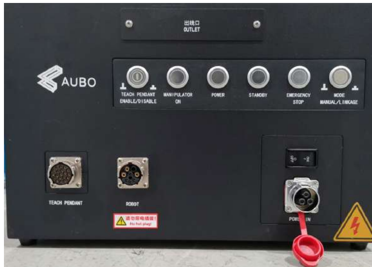
Figure 7-2 Front panel of the control box
